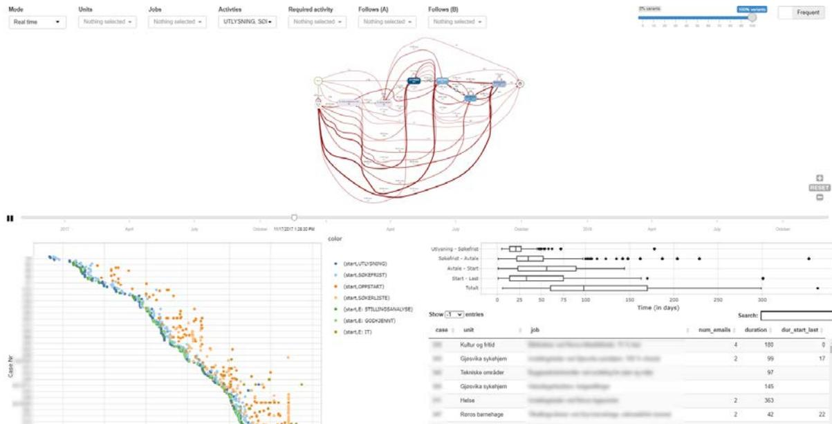
Figure 4. Screenshot of the developed Process Mining dashboard: the top part shows the process map visualisation, the lower left part shows a dotted chart visualisation, and the lower right part shows an interactive table of process cases.
