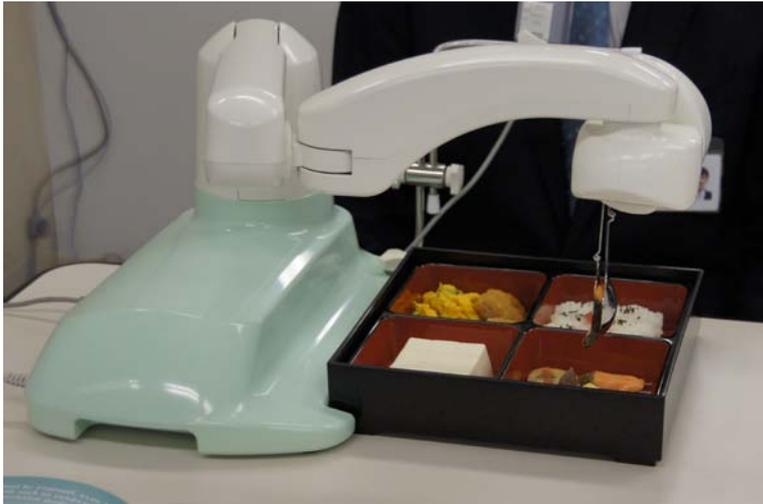
*Figure 3. The Secom manufactured My Spoon feeding robot*
