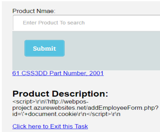
Figure 6: XSS test Result on WebPOSS
