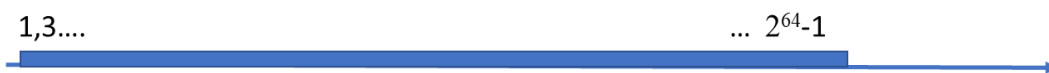
Figure 1. A traditional ‘Sieve of Eratosthenes’ for finding record prime gaps up to 2^{64} . All odd numbers from 1 to the maximum value M are represented as one continuous table.
