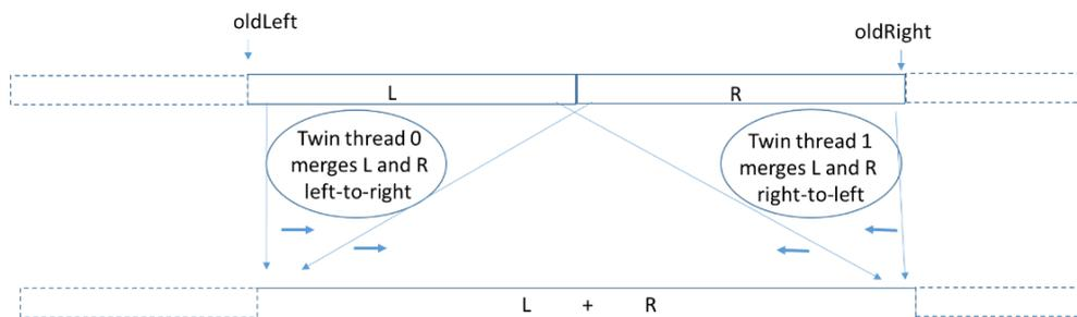
**Figure 1.** Merging adjacent sorted sections  $L$  and  $R$  in parallel with two twin threads – each merging number of elements = half the sum of the length of  $R+L$ . Thread<sub>0</sub> merges  $L$  and  $R$  from **left** to **right** on smallest elements, while thread<sub>1</sub> merges  $L$  and  $R$  from **right** to **left** on largest elements.
