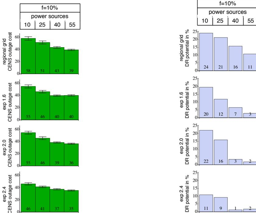
(a) *CENS* outage cost in the regional grid and in random networks whose node degrees follow an exponential distribution  $exp(\lambda)$  with  $\lambda \in \{1.6, 2.0, 2.4\}$ . The repair strategy *Minimize CENS* is used after 10% of the nodes failed. The non-alive nodes are determined with the *Balancing* measure. Whiskers indicate the standard error of mean.
